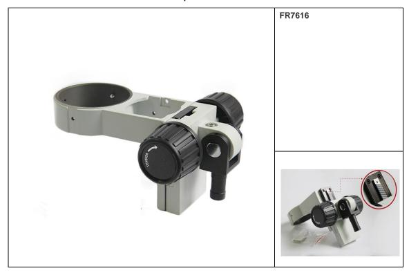
E-Arm Focus mount with 76mm diameter ring with 15.875mm (5/8") adapter can be mounted on any of our boom stands or articulating arm stands, and features Rack & Pinion coarse focus adjustment. 50mm focusing distance in vertical direction.
