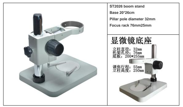
boom stand heavy metal base Stereo Microscope Bracket Plane frames, Steel Rail Rack Focusing Mechanism Connectiong Objective: DIA 76mm Connectiong Pillar: DIA 32mm Size of Pedestal: 255 x 200 x 24mm Easy Large-Sized Focusing Knobs on Both Sides of Focusing Holder. Steel Gears on Focusing Holder. Standard Size Focusing Holder - Will Fit Scope Heads with Diameter of 76mm
